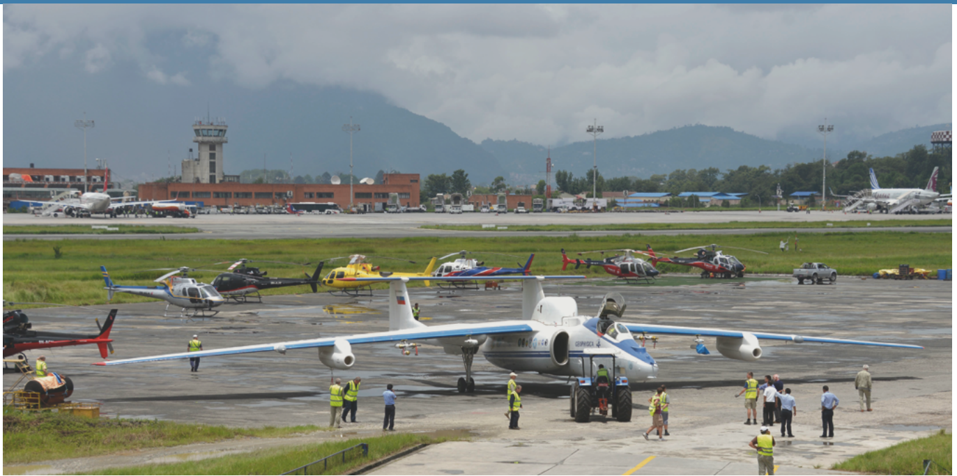
Fig. 1: The single-seated research aircraft M55 Geophysica can fly at altitudes exceeding 20 kilometres. Here it is prepared at the airfield in Kathmandu in July 2017 to conduct the first measurement flights to the stratosphere in the Asian monsoon region. On board: the instrument HAGAR ("High Altitude Gas Analyzer") operated by the University of Wuppertal team to analyse the air for CO 2 , N 2 O, CFCs and other long-lived trace gases.
