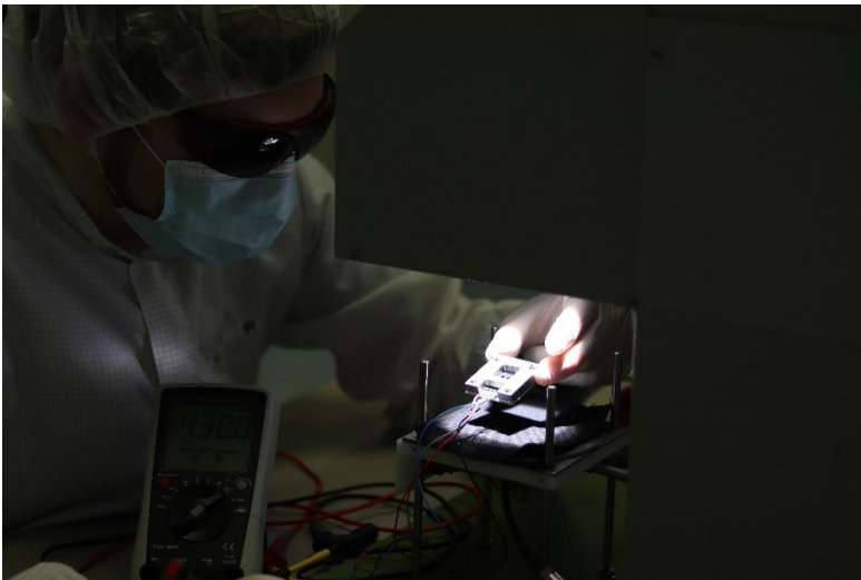
Measurement of a tandem solar cell under a solar simulator. // picture: Cedric Kreusel
